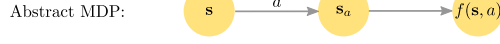
(b) Modified MDP model that is used to encode safety features that depend on actions. In this model, actions lead to abstract action-states s_a , which only have one available action that leads to f(s, a) .
