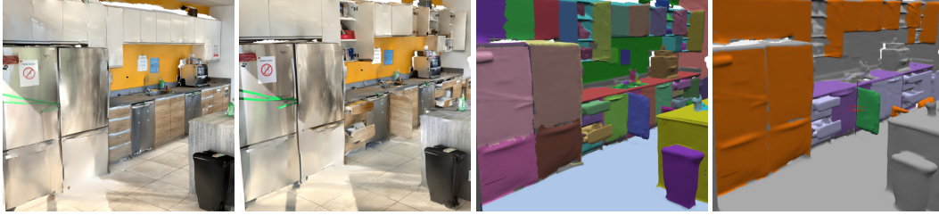
Figure 10: Left and middle left: two scans of a kitchen in different states. Middle right: part-level semantic instance annotation of objects and their parts. Right: articulated parts highlighted in color.
