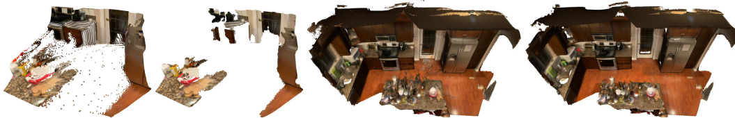
Figure 2: Depth map filtering. From left: raw acquired depth map, filtered depth map, reconstruction result with raw depth maps, reconstruction result with filtered depth maps. Filtering of low-confidence and rapidly changing depth values leads to fewer floating point artifacts.
