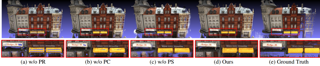
Figure 5: Reconstruction results of ablation study on part-aware patchmatch, without part representation (w/o PR), part-aware correspondence (w/o PC) and part smoothness (w/o PS) relatively.
