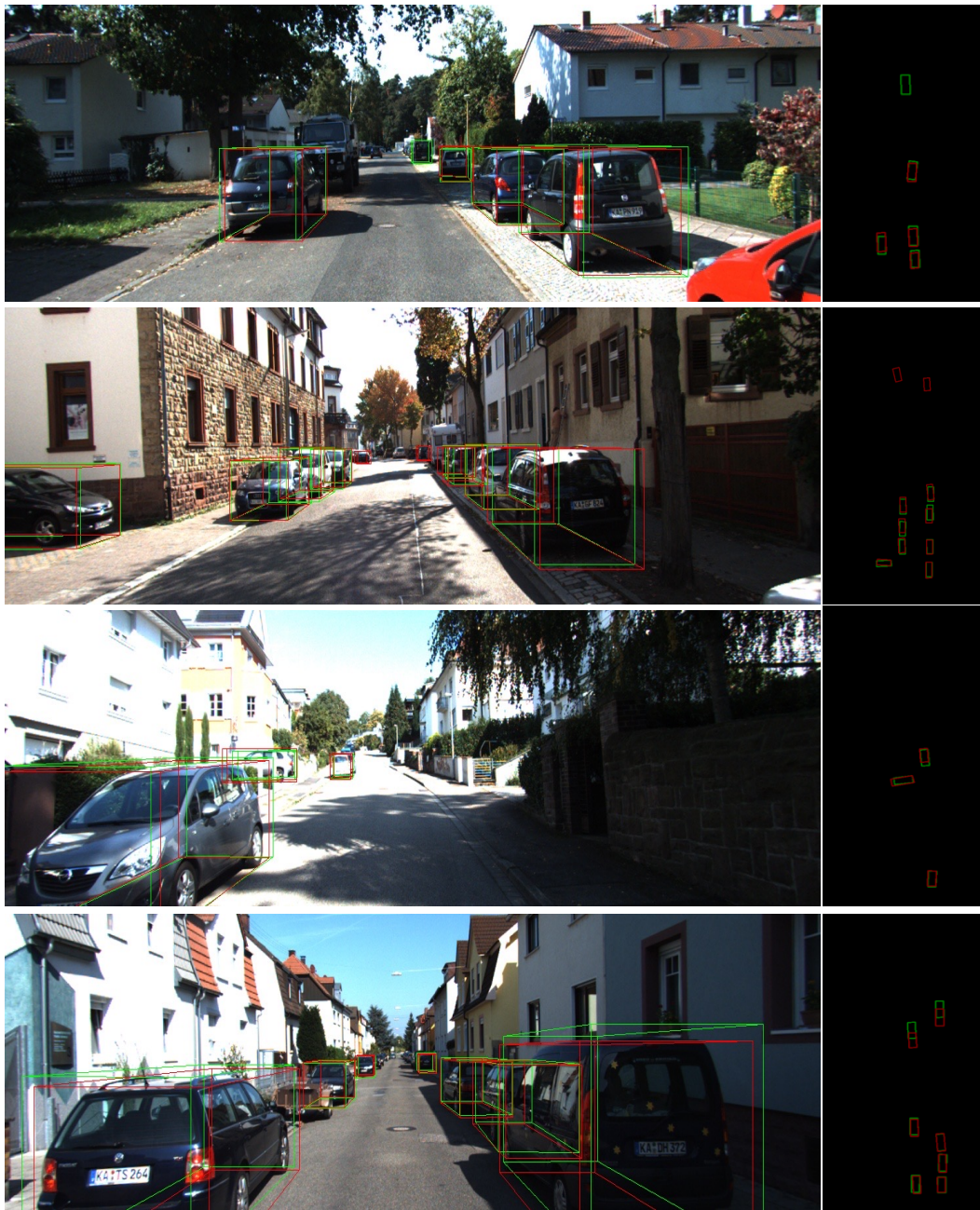
Figure 3: Qualitative Results on KITTI. The 3D green boxes are produced by MonoUNI and the red boxes are the ground truths.
