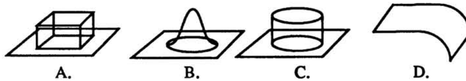
Figure 3: Internal bump functions for A) oct-trees, kd-trees, boxtrees (Omohundro, 1987), B) and C) for balltrees (Omohundro, 1989), and D) for Sproull's higher performance kd-tree (Sproull, 1990).
