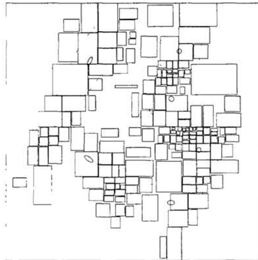
Figure 3: The ellipses show the model \theta^t at the start of an EM iteration. The rectangles depict the mrkd -tree nodes that were pruned. Observe larger rectangles (and larger savings) in areas with less variation in class probabilities. Note this is not merely able to only prune where the data density is low.
