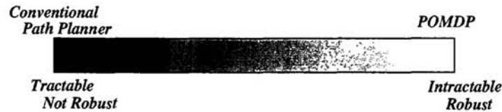
Figure 1: The continuum of possible approaches to the motion planning, from the robust but intractable POMDP, to the potentially failure-prone but real-time conventional planners. Coastal navigation lies in the middle of this spectrum.
