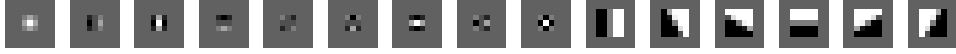
Figure 1: The convolutional filters used for texture energies and gradients. The first nine are 3x3 Laws' masks. The last six are the oriented edge detectors spaced at 30^\circ intervals. The nine Law's masks are used to perform local averaging, edge detection and spot detection.
