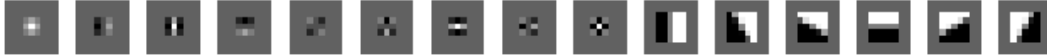
Figure 2: Examples of different edge and texture filters used to calculate the features.
