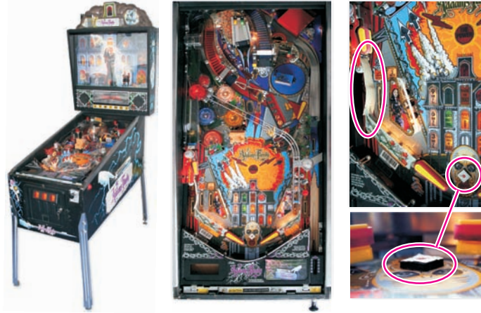
Figure 1: Left: pinball machine used for the present study. Middle: Close look at the build-in gadgets of the play field. Right: Zoom into the modified parts of the play field (side walls and central bump).
