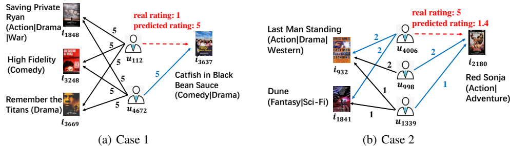
Figure 3: A case study of debugging wrong prediction by generating intuitive explanations. Movie titles and genres are also shown. The red dashed line is the inaccurate prediction to debug, and the solid lines are the corresponding explanations. For example, in the left case, “5 stars” rating from user 4672 to item 3637 (the blue solid line on the right) is most responsible for the wrong prediction (the red dashed line).
