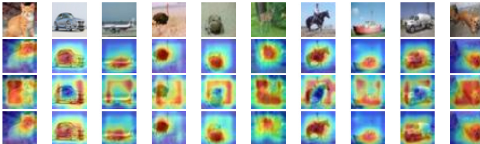
Figure 4: Feature map visualization of WideResNet-40-4. The top row is the original image, and the feature maps of the baseline model, pruned model, and merged model are in order. We select one image for each image label.
