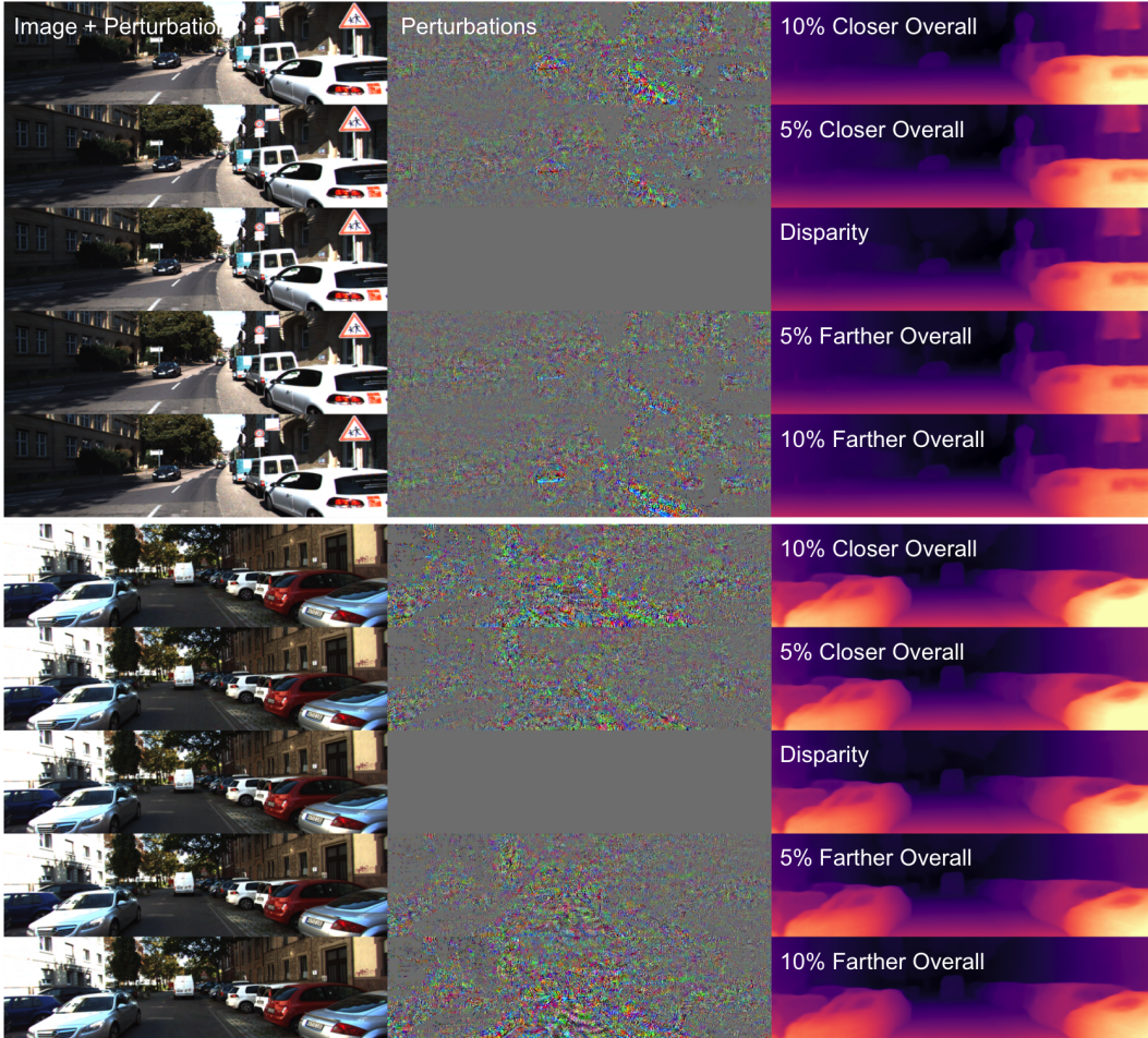
Figure 11: Visually imperceptible perturbations v(x) , with \xi = 2 \times 10^{-2} , can fool Monodepth2 to predicted scenes that are 5% or 10% closer and also 5% or 10% farther.
