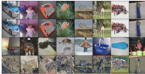
Figure 7: Analysis of the HF content in C' for R revealing the secret image. The four rows from top to bottom indicate C' , C' with HF content filtered out, S and revealed S' with filtered C' .
