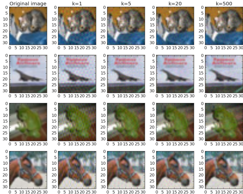
Figure 3: Original images (leftmost) from the CIFAR-10 dataset and their perturbed versions when sparse random perturbations are added in the DCT basis with sparsity k . Large perturbations in the DCT basis (e.g., k = 1 ) lead to perceptible changes in the pixel space though they are \ell_\infty perturbations of \varepsilon \leq 0.09 . As k increases the imperceptibility of the perturbed images improves.
