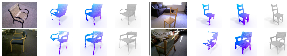
Figure 11: Tests on real scans [6]. From left to right: image of the target object; input partial scan; predicted point cloud; predicted 3D mesh.
