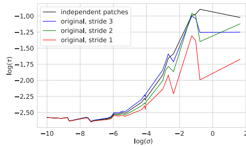
Figure 22: f(\sigma) curve for training on random labels with different approximations of CIFAR10 images. Two 3 \times 3 -convolutional layers, one fully connected layer. Correlations between neighboring patches create deviation from the curve seen for the “ideal” case of independent Gaussian approximations. Smaller strides lead to stronger correlations and stronger deviation.
