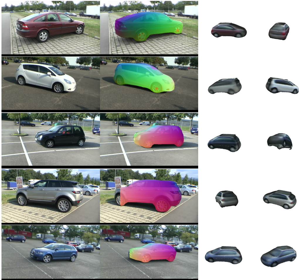
Figure IV: Additional single-view reconstruction results on images from the test sequences of Freiburg Cars. Columns: input image; canonical mapping; 3D reconstruction with the reconstructed texture from two viewpoints.
