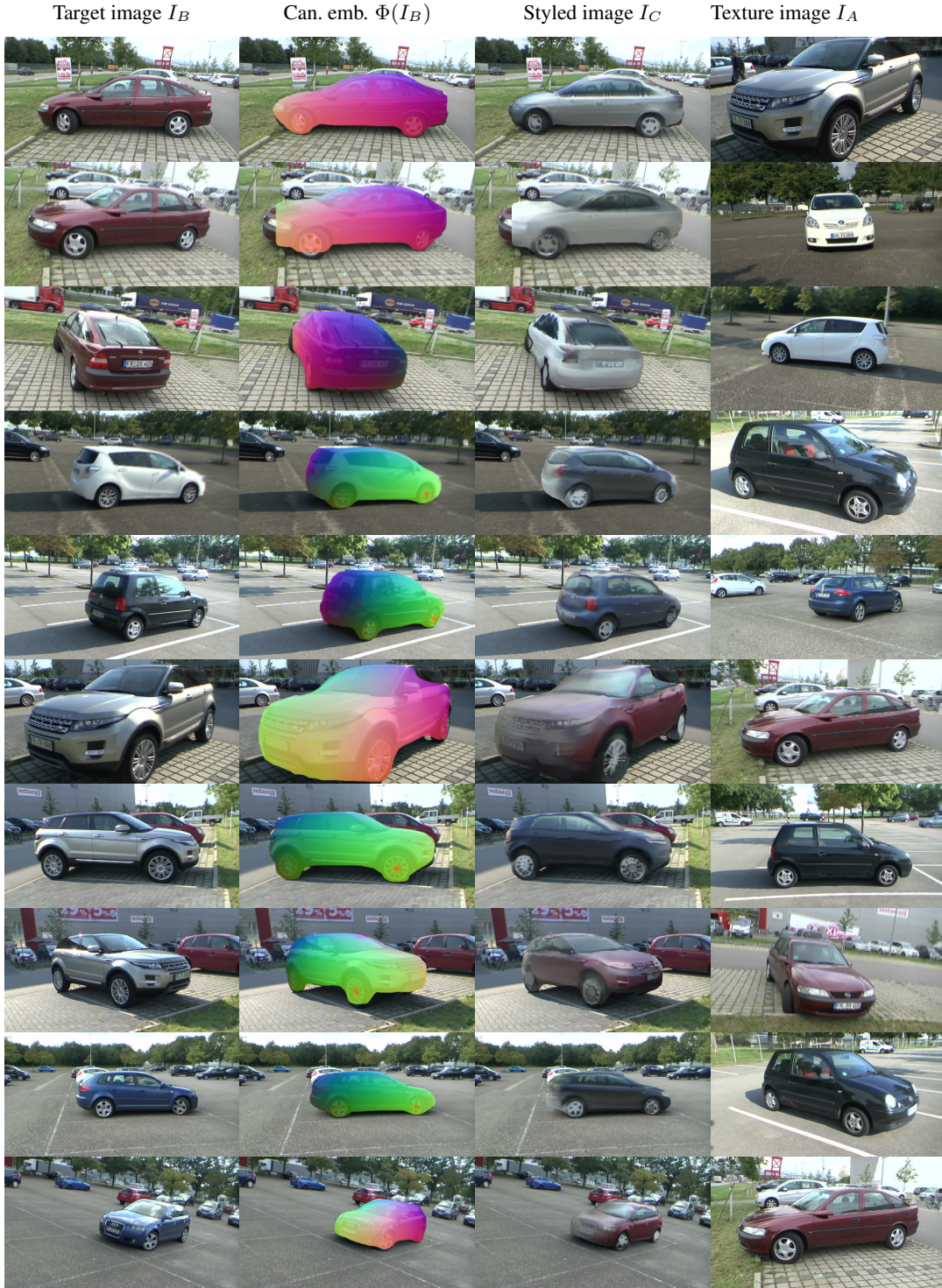
Figure VI: Canonical mapping and texture transfer for Freiburg cars. Given a target image I_B (1 st row), C3DM extracts the canonical embeddings \kappa = \Phi(\mathbf{y}; I_B) (2 nd row). Then, given the appearance descriptor \beta(I_A) of a texture image I_A (4 th row), the texture network C transfers its style to get a styled image I_C(\mathbf{y}) = C(\Phi_{\mathbf{y}}(I_B); \beta(I_A)) (3 rd row), which preserves the geometry of the target image I_B .
