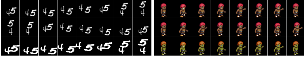
Figure 2: Data augmentations on SM-MNIST and Sprites. Left panel: SM-MNIST. The first row is the raw input sequence of moving digits. The second row reverses the sequence order of the raw sequence, serving as the content augmentation. The third row stretches the frames and enhances the color, which changes the digit styles but does not change the digit movements and thus forms a motion augmentation. Right panel: Sprites. The first row is the raw input character video. The second row is the content augmentation with a random order. The third row is a motion augmentation produced by distorting colors and adding Gaussian noise.
