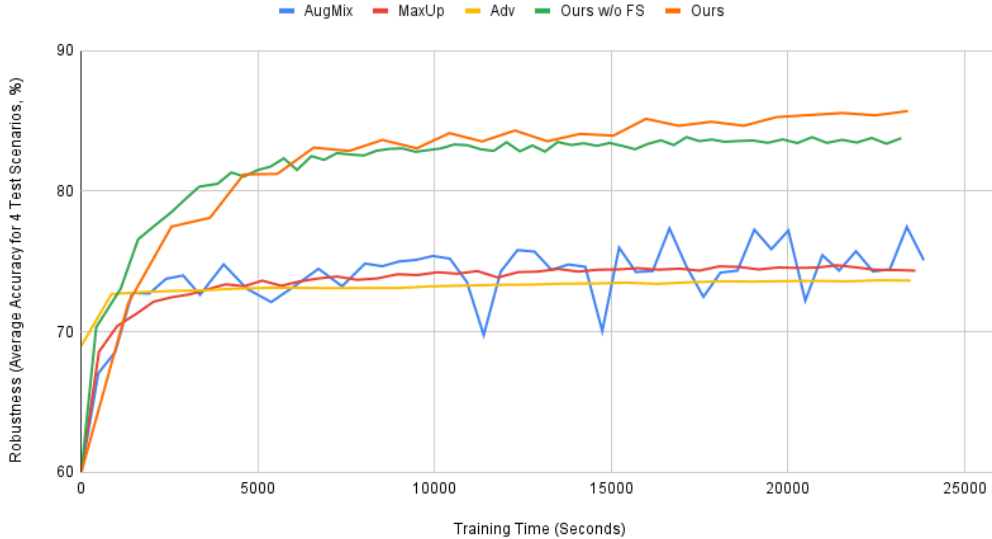
Figure 4: Efficiency comparison between our method and other SOTA methods with the Nvidia Network [4] on the SullyChen dataset [7]. The x-axis is training time (in seconds), while the y-axis displays overall robustness, i.e., the average accuracy of the 4 test scenarios (clean, single perturbation, combined perturbation and unseen perturbation). Our method outperforms other methods with higher accuracy and better efficiency. For example, after 1/10 the training time (2500 sec), our performance is already better than others’ final performance (after 25,000 sec of training).
