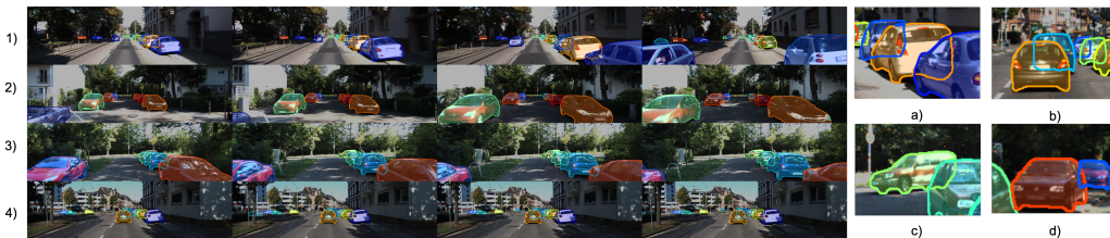
Figure 3: Visualization of the prediction of our SaVos model on KINS-Video-Car dataset. The transparent mask is the predicted modal mask by PointTrack[6]. The solid curve are the contours of the amodal prediction by SaVos. From the figure we can see our model can predict the amodal mask well in the scene with multiple cars and heavy occlusion. Our model performs well for cars in different viewing angles and occlusion patterns. For examples: a)-d), which are cropped from the case 1)-4), respectively.
