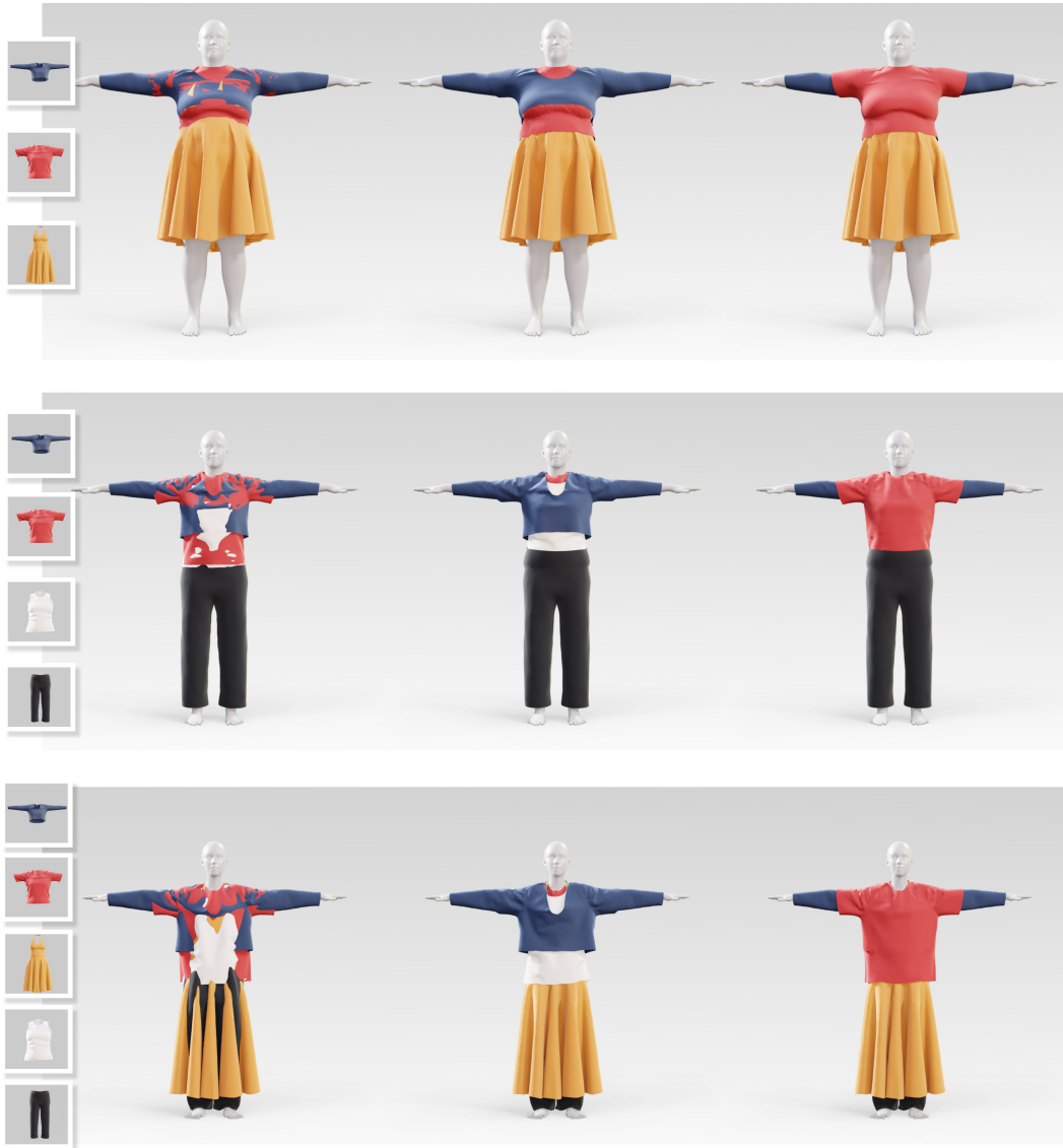
Figure 3: Given a set of garments (left insets), existing VTO methods [57] infer their fit into a target body shape but produce a heavily entangled results (left). In contrast, ULNeF untangles the garments by directly projecting their neural fields into a collision-free configuration. Since ULNeF allows to specify the desired order, different outfits can be created (center and right).
