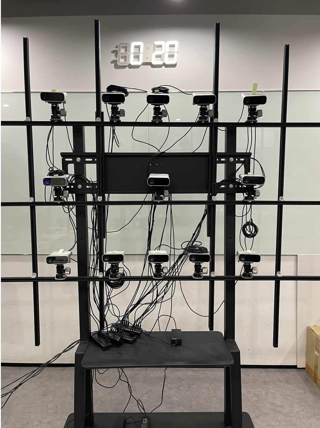
Figure 1: The multi-camera capture system.
