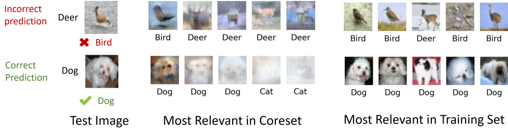
Figure 6: The most relevant images for an incorrect (top row) and correct (bottom row) prediction on CIFAR-10. The most relevant coreset images are picked based on the coreset influence score I , and for their training set, the training influence score J . These metrics are fast to compute and result in semantically meaningful explanations for these two predictions.
