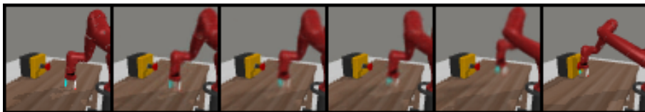
Figure 10: Example of invalid image sequence (left to right) planned with HTM . Sequence contains shortcut connection between the last two frames.
