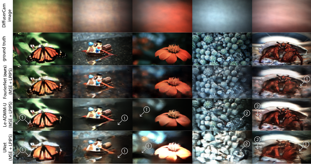
Figure 2: Comparisons of our method (third row) to state-of-the-art learned reconstruction methods on lensless diffused images of natural scenes. Regions labeled ① indicate missing details, either resolution or textures in backgrounds. Regions labeled ② indicate hallucinated textures. Note that the previous state-of-the-art solution (fourth row) [25] exhibits both issues more often compared to our method.
