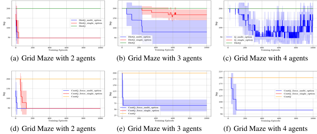
Figure 5: Evaluation on n -agent Grid Maze tasks: (a)-(c): Distributed Q-Learning; (d)-(f) Centralized Q-Learning + Force. The performance improvement of our approach are more and more significant as the number of agents increases. The centralized way to utilize the n -agent options performs better.
