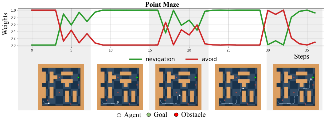
Figure 3: Weights inference over one episode (Point Maze). ASPiRe is able to compose the navigation prior and avoid prior concurrently (grey phases) when the obstacle is observed and only activate navigation prior when it is not (white phases).
