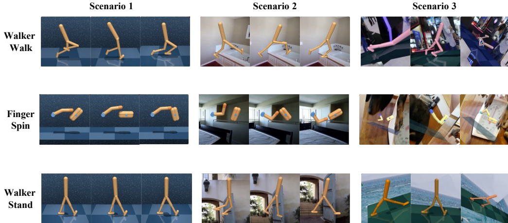
Figure 25: Visualization of three trained tasks in different visual scenarios. The scenario 1 is constructed in a static and clean visual scenario. Conversely, the scenario 2 introduces dynamic variations by employing a video background that alters with each episode, encompassing a total of 110 distinct videos. The scenario 3 further extends this complexity by incorporating additional visual generalization types, such as changes in camera view and lighting conditions.
