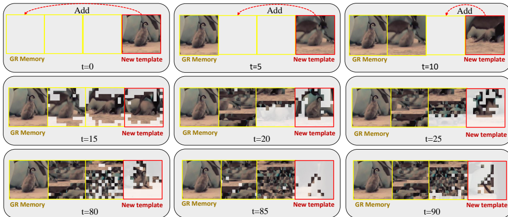
Figure 5: Visualization of GR memory updates. Over time t , the GR memory accumulates an increasing number of representative penguin features. In the second and third rows, white tokens represent discards, while the other tokens are retained in memory.
