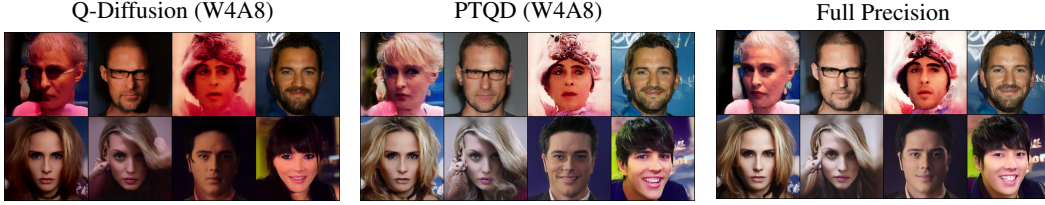
Figure 1: The comparisons of samples generated by Q-Diffusion [31], PTQD and full-precision LDM-4 [45] on CelebA-HQ 256 \times 256 dataset. Here, WxAy indicates the weights are quantized to x -bit while the activations are quantized to y -bit.
