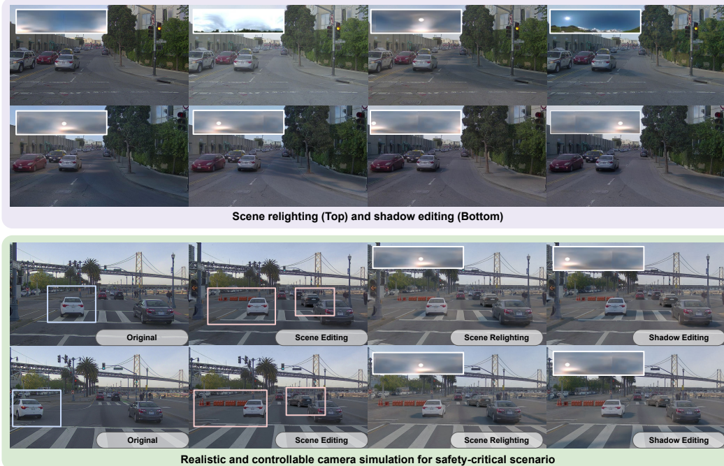
Figure 1: LightSim builds digital twins from large-scale data with lighting variations and generates high-fidelity simulation videos. Top: LightSim produces realistic scene relighting and shadow editing videos. Bottom: We generate a safety-critical scenario with two vehicles cutting in and perform lighting-aware camera simulation. See Appendix E and project page for more examples.
