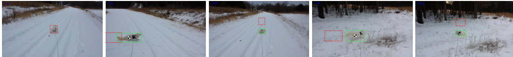
(f) fox-2. Special case . Though the background is pure white, the target object is also white. In this case, lost tracking happens.
