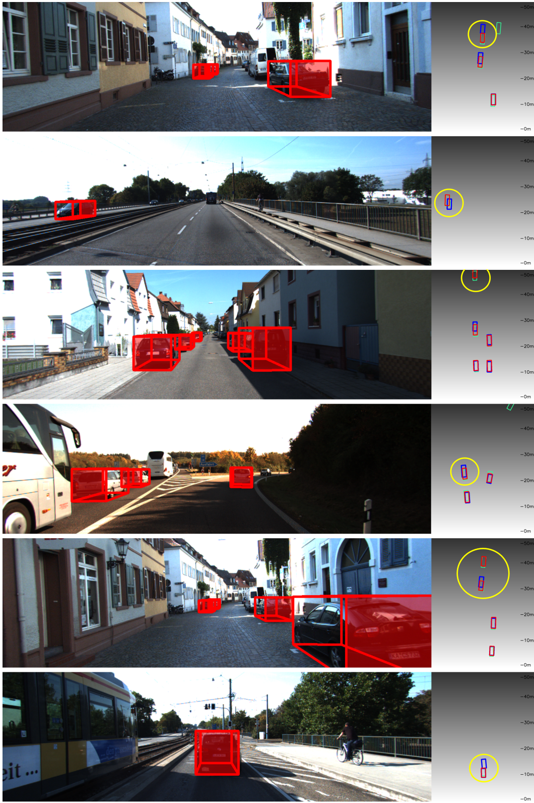
Figure 2: Comparison of qualitative results between MonoCon and MonoCon + ours. Yellow circles highlight accurately estimated parts compared to the MonoCon. (GT: green, Prediction of MonoCon: blue, Prediction of MonoCon + Ours: red)
