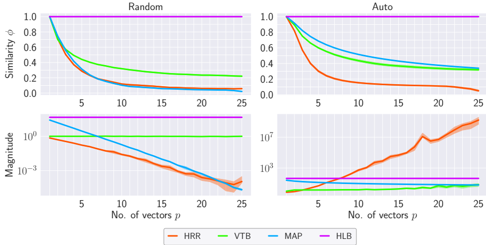
Figure 3: When repeatedly binding different random (left) or a single vector (right), HLB consistently returns the ideal similarity score of 1 for a present item (top row) and has a constant magnitude (bottom row), avoiding exploding/vanishing values.
