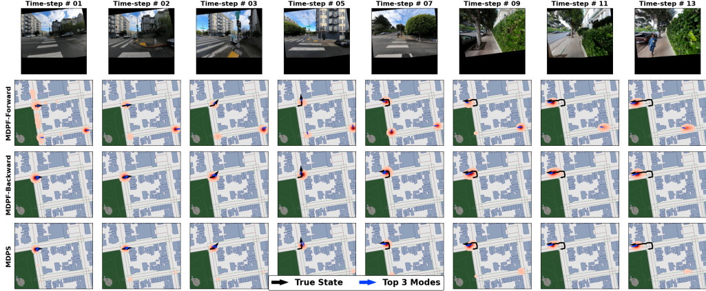
Figure 4: Example trajectories from the MGL dataset with observations shown in the top row. We show the current true state and state history (black arrow and black line), the estimated posterior density of the current state (red cloud, with darker being higher probability) and the top 3 extracted modes (blue arrows) for the MDPS as well as its forward and backward MDPFs. Due to ambiguity at early time-steps, MDPF [14] is unable to resolve the correct intersection, and instead places probability mass at multiple intersections. By fusing both forward and backward filters, our MDPS resolves this ambiguity with probability mass focused on the correct intersection. Furthermore, MDPS provides a tighter posterior density than either MDPF-Forward or MDPF-Backward.
