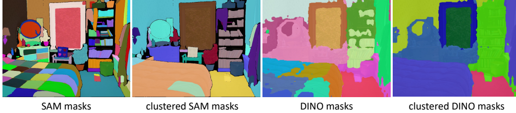
Figure 2: Visualization of masks from vision foundation models. We visualize the masks generated by SAM [13] and by clustering image features from DINO [14]. Although such models can freely generate fine-grained masks, the resulting masks can be too small or incomplete to have semantic meaning. To address this over-segmentation issue, we employ online clustering [18] of the masks into semantically meaningful groups defined globally for given images.
