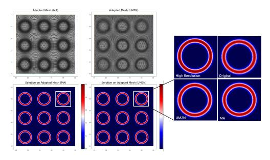
Figure A3: Visualization of UM2N output mesh and reference mesh from MA. Comparison between solutions obtained on high resolution, original, UM2N and MA meshes.
