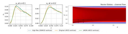
Figure A4: Boundary Layer. The two plots at left visualize the  $u_y$  from boundary to y = 0.1. It can be observed that UM2N improves the accuracy of the velocity obtained on uniform mesh compared to High Res solution.
