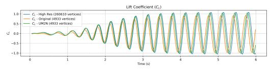
Figure A10: Results of  $C_L$  coefficients. The blue, orange and green lines show the drag  $C_L$  coefficients obtained on a high resolution fixed mesh, UM2N adapted mesh and the original coarse mesh for the first 6 seconds (i.e., 6000 steps). It can be observed that the UM2N output mesh improves the accuracy of  $C_L$  in magnitude and periodicity compared to the original mesh.
