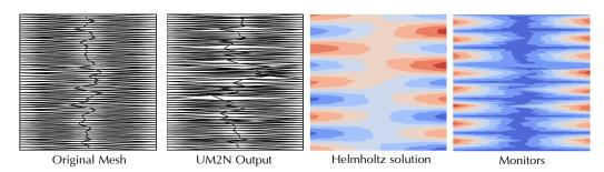
Figure A5: A very poor initial mesh case. UM2N perform mesh movement for an anisotropic Helmholtz problem.
