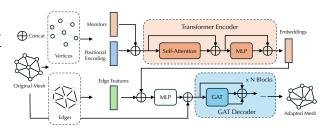
catenated with the extracted edge features *e* to serve as the input for the Graph Attention Network (GAT) decoder. The decoder processes this combined input along with a mesh query to ultimately produce an adapted mesh.
