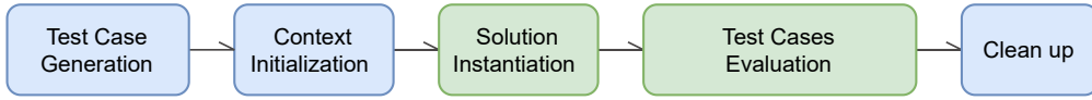
Figure 5: Sandbox Execution Pipeline. 1) Test Case Generation. We first employ the corresponding test case generator for each task to produce a comprehensive set of test cases for the subsequent evaluation. 2) Context Initialization. To prevent any unexpected code behavior, the sandbox environment is meticulously reinitialized for each new task. This phase ensures that all the common libraries required for executing the solution are loaded. 3) Solution Instantiation. The solution under evaluation will be encapsulated as a solution class. 4) Test Case Evaluation. Each test case the generator provides will be rigorously executed against the solution. A solution must successfully pass all the test cases to be deemed valid. 5) Clean up. The final stage involves the sandbox dutifully clearing the namespace environment and the temporary directory. Mercury records the time consumed during the stage of Solution instantiation and Test Ease Evaluation as the primary metric for assessing code efficiency.
