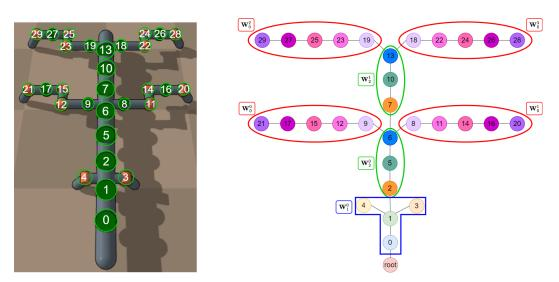
Figure 20: Graph Structure and Modules of the 6 Leg Hybrid. Left: Rendered robot, with joints labeled numerically and circled. **Right:** Corresponding graph structure with joints as nodes and links as edges. The joints circled in red belong to the "leg" modules, those circled in green belong to "body" modules, and those circled in blue belong to the "head" module.
