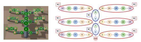
Figure 1: Graph Structure and Neural Network Modules of the 6 Leg Centipede. Left: The robot's joints are labeled numerically and circled. Right: The joints form the nodes and the links are the edges. The subset of joints that form each leg module are circled in red, while those that comprise each body module are circled in blue. Neural network modules are denoted as  $W_k^i$ , where k refers to the type, e.g. all leg modules are type 0, and i denotes different instances of the same module type.
