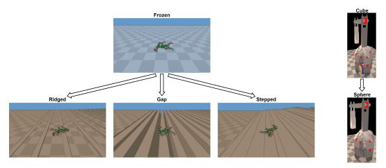
Figure 18: **Task transfer. Left:** The training task is a 6 leg centipede locomoting over the Frozen Terrain. The goal is to transfer policy weights to Ridged, Gap, and Stepped Terrains, all of which require the robot to overcome obstacles unseen in the Frozen Terrain. **Right:** In the grasping domain, the training task is a 4 finger claw lifting a cube, and the testing task is the same claw lifting a sphere. A sphere is naturally a harder object to grasp due to its curved surface.
