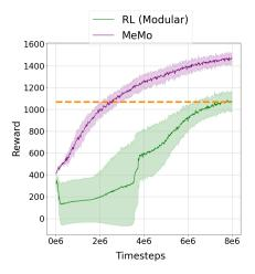
Figure 13: 6 Leg to 24 Leg Centipede Transfer Results. The dashed orange line shows that the final performance of the closest baseline is achieved by MeMo in less than half of the total number of timesteps.
