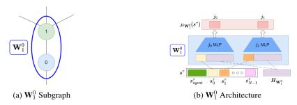
Figure 11: Module Subgraph and Architecture. Left: Module  $W_1^0$  is responsible for computing the mean actions of actuators 0 and 1. Right: A module consists of separate networks that compute each actuator's mean action. The inputs include the local observations of the actuator concatenated with the signal sent to the module it belongs to.
