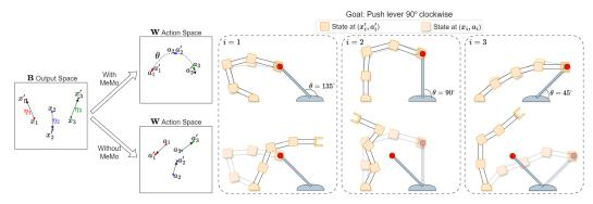
Figure 2: Effect of Modularity Objectives. Consider a module with 5 actuators, denoted in orange, trained to push a lever clockwise. As the state of the lever is a function of its angle  $\theta$ , a module trained by MeMo represents the control signals as a one-dimensional manifold with respect to **B**'s signal. When noise is added to **B**'s signal, the outputted actions remain on the manifold. Without MeMo, perturbations to **B**'s signals cause deviations from the high reward trajectory.
