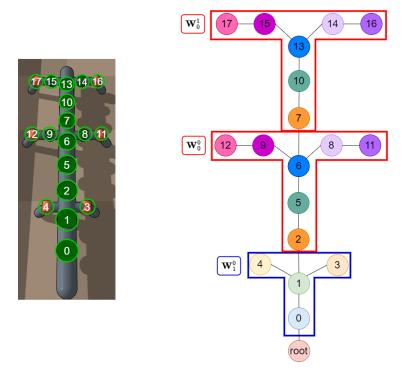
Figure 19: **Graph Structure and Modules of the 6 Leg Worm. Left:** Rendered robot, with joints labeled numerically and circled. **Right:** Corresponding graph structure with joints as nodes and links as edges. The joints circled in red can be thought of the "head" while the joints circled in blue form the "body" modules.
