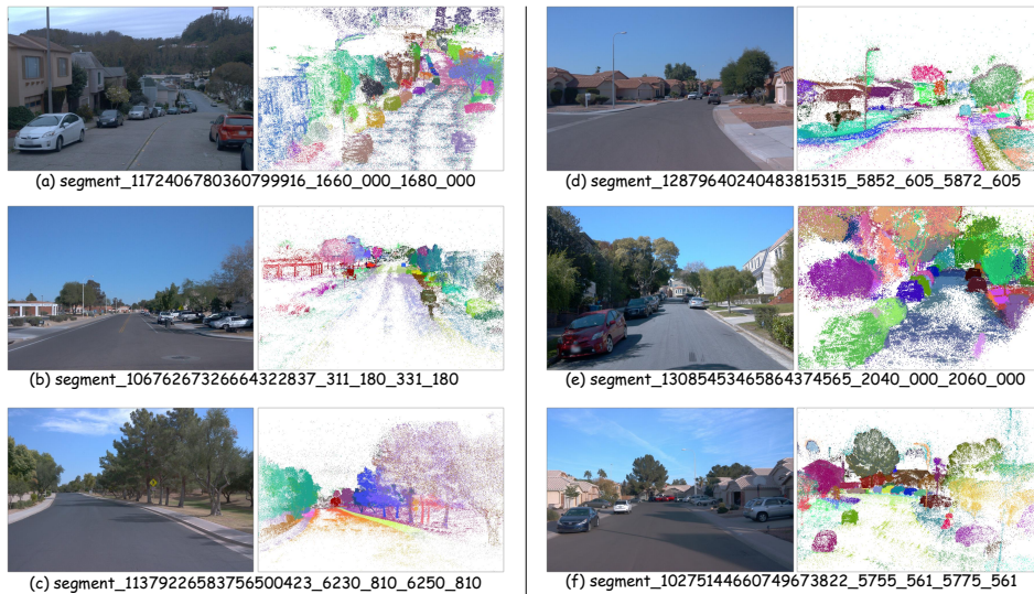
Figure 13: Feature visualization of 3D points on the large-scale outdoor dataset Waymo. (a)-(f) are 6 different scenes selected from the Waymo dataset. Left: RGB image; Right: 3D point features.
