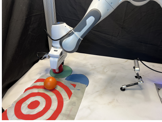
Figure 16: We randomly throw a target bag on the table as a strong visual distractor. Diffusion Forcing can be prompted to treat observation as corrupted rather than ground truth.
