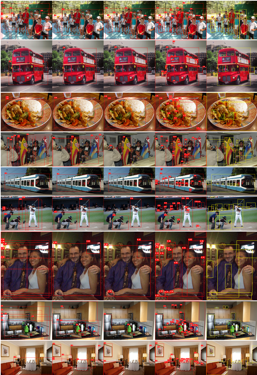
Figure 9: Additional visualizations of class-agnostic box predictions. Columns 1 – 4 correspond to the following methods: MOST [43], CutLER [50], zero-shot Grounding DINO [“generic”] [9], and our proposed DiPEx, respectively. The final column presents human-annotated ground truth bounding boxes from the MS-COCO dataset [32].
