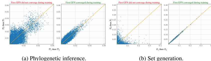
Figure 8: Permutation invariance of SB-GFlowNets for phylogenetics (a) and set generation (b). When the first GFlowNet is not adequately trained, the learned distribution after two streaming updates depends on the ordering of the observed datasets ( left (a), left (b)). In contrast, when both the first and second GFlowNets are accurate, the resulting distribution is approximately invariant to the data permutation ( right (a), right (b)).
