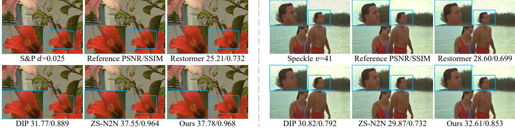
Figure 6: Qualitative results on unseen noise types. Restormer is trained with Gaussian \sigma=25 . Noisy patches are from kodim07 and kodim12.
