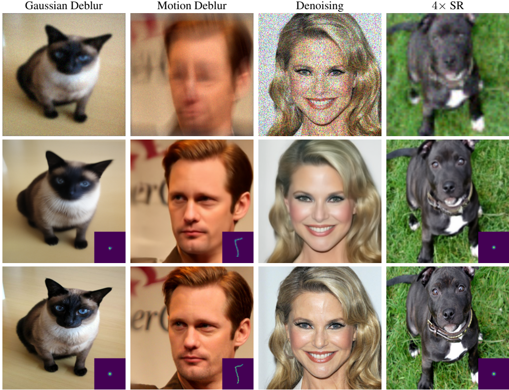
Figure 2: We demonstrate BIRD on several blind image restoration problems ( i.e. , when the values of the degradation model are unknown): Gaussian deblurring, motion deblurring, superresolution (SR) (it includes additional Gaussian blur) and denoising with an unknown noise distribution. BIRD is applicable to a single degraded image and does not require re-training or fine-tuning of the prior model (we use a diffusion model). Although some of the generated degraded images use Gaussian blur, BIRD recovers a generic blur kernel (without making any Gaussianity assumption).
