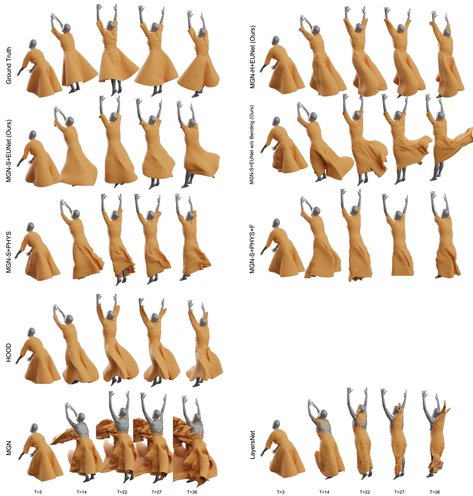
Figure 9: We display the qualitative results for all models. Simulators constrained by our EUNet deliver dynamic patterns closer to the ground truth. We further demonstrate the effectiveness of the bending forces captured by our EUNet, which is shown on the second row. Without the bending forces, the MGN-S+EUNet tends to generate more wrinkles but different deformation patterns as the ground truth garments.
