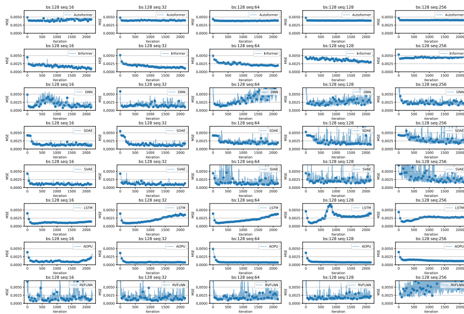
Figure 10: Curves of SRU validation loss changes with training iteration for different models with fixed batch size of 128 at different sequence length settings.
