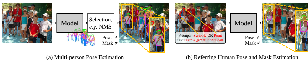
Figure 1: Task illustration of (a) multi-person pose estimation predicts numerous outcomes and requires selection strategies during deployment, potentially leading to false negatives or suboptimal target results, and (b) our referring human pose and mask estimation requires a unified promptable model to simultaneously predict accurate pose and mask for the person of interest, providing comprehensive and identity-aware human representations to benefit human-AI interaction.
