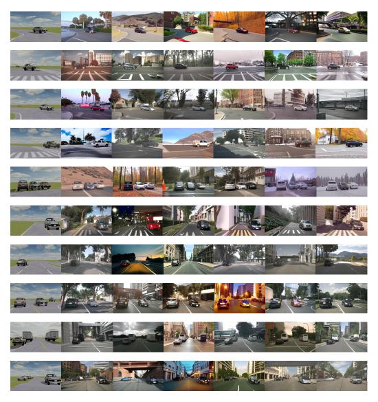
Figure 15: **Diverse generated images from simulator scenarios** From the same original simulated driving scenario (left column), we show a diverse range of generated images (columns 2 through 7). SimGen is capable of generating driving scenes in a wide variety of settings based on the same simulator conditions.
